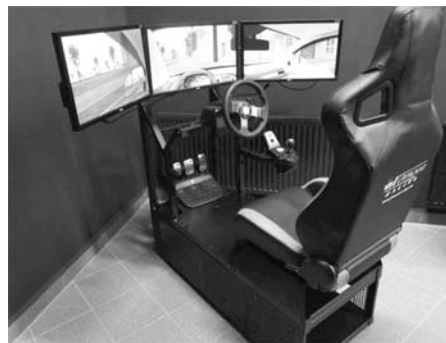
Fig. 3. A simplified driver station. Source: Obtaining data from the privileged vehicles driving simulator.
