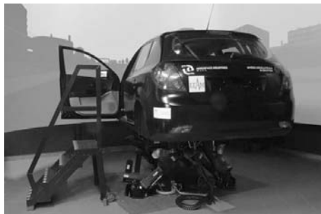
Fig. 1. A cabin of the car with the motion system. Source: Obtaining data from the privileged vehicles driving simulator
